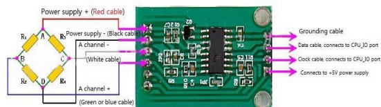
Gambar 2.8 Penggunaan HX711 Sumber : ( Principle and Usage of HX711 Weighing Sensor Module , 2014)
