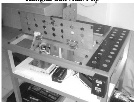
Gambar 19. Hasil Realisasi Rancangan T-Shirt Folding Machine
